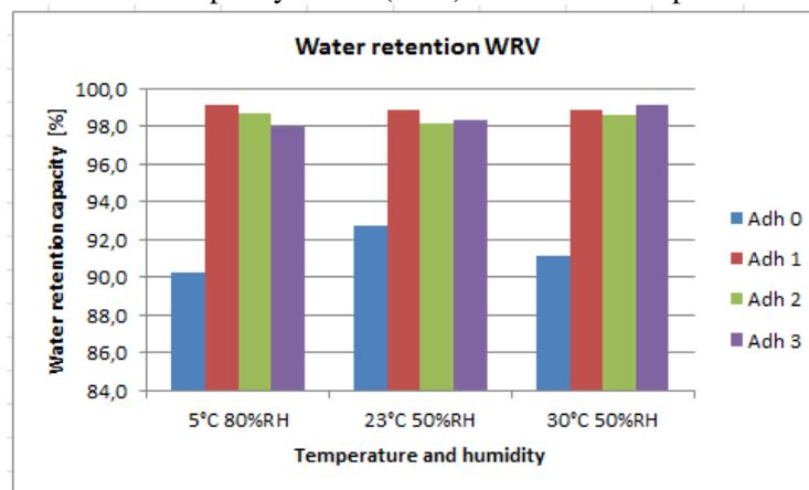
Before the test materials were stored in various appropriate conditions. Mortar without cellulose ethers kept the water at about 91% and the other materials at about 98%. At this thickness, in such a short time, the effect of temperature was small.
